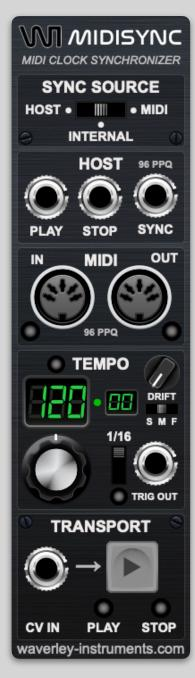
MIDISYNC is a MIDI clock synchronisation utility module for Voltage Modular that can be used in a number of ways.
