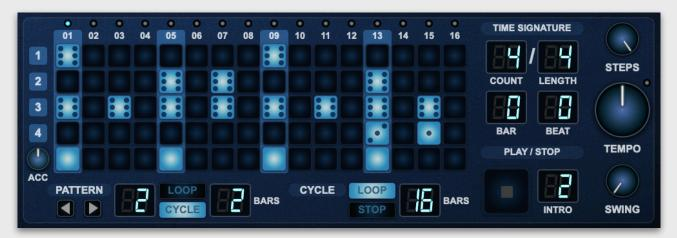
The sequencer is a traditional four lane 16 step pattern sequencer, each voice having its own dedicate lane or track. An additional lane allows accents to be added for certain steps and the accent is applied to all voices for that step according to the level of the ACC control.
